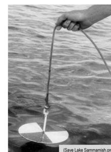
Figure 4: Secchi Disk
